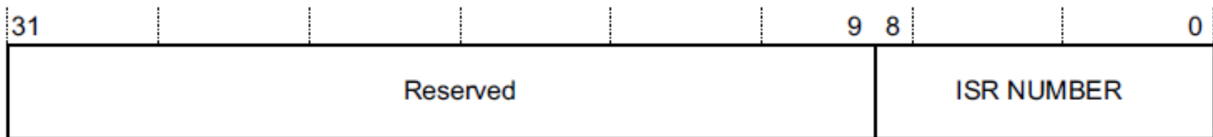
Figure 2-3 Interrupt Program Status Register bit assignments
